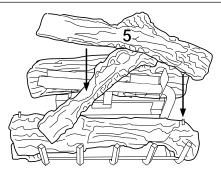
Figure 44 - Installing Log No. 5
